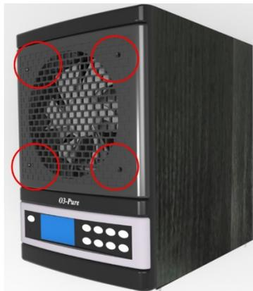
Note: It is normal for the ANION to cause some particles to accumulate on the front grill and fan blades. Use a Phillips-head screw driver to remove the (4) screws in the front grill cover. Simply clean the blades and grill with a damp cloth or vacuum. Allow to dry completely before re-attaching the front grill cover.
