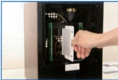
Remove the Pre-Filter, the HEPA filter, the Activated Carbon and Photo-Catalytic filters. Carefully remove the white purification plate by grasping the end and carefully pulling straight out of the card slot. Clean the plate
