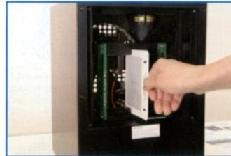
6. Reinstall the 3 inner filters in the following order:
